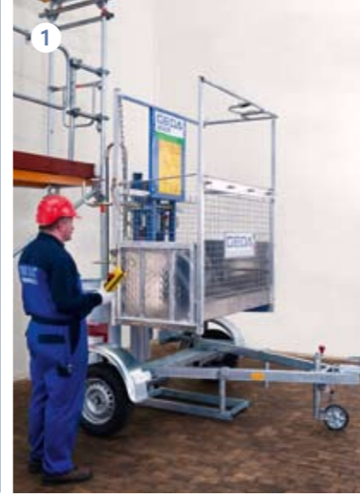
1 Automatic unloading from the trailer.
